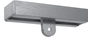
Fig. 170 Horizontal Traveler Size Range: Available in four sizes to take loads to 20,700 (lbs.) All sizes provide for 12" of horizontal travel. Page 184
