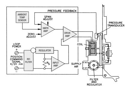
The Apex 5100 I/P Module converts 4-20 mA current signals into 3-15 psi pneumatic signals needed by the Apex 5000 Positioner. A controller card compares the input signal with an electrical pressure feedback signal and outputs voltage, which is applied to a coil.
