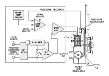
The APEX 6100 I/P module converts 4-20 mA current signals into 3-15 psi pneumatic signals needed by the APEX 6000 positioner. A controller card compares the input signal with an electrical pressure feedback signal and outputs voltage, which is applied to a coil.
