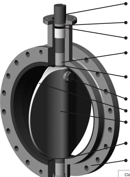
K-Flo 500 series valves feature a one-piece-throughshaft design for high strength and positive disc control. The shaft meets or exceeds all requirements of AWWA C504 Class 150B.
