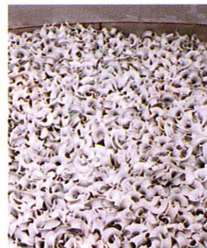
3" saddles loaded in an Absorbing Tower
