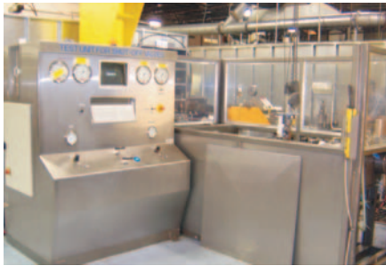
Every Orbit valve is individually pressure tested to meet or exceed industry standards.
