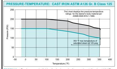
**TESTING:** Strainers are individually, hydrostatically tested at 1.5 x the 100  $^{\circ}$ F rating, rounded off to the next higher 25 PSI measurement .
