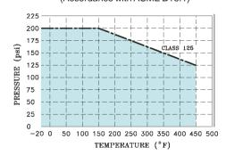
Lower Temperature Limit -20°F/-28.9°C M.A.W.P. - Nonshock 2"-12" 200 psi/13.7 bar 14" and up 150 psi/10.34 bar
