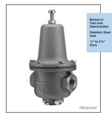
The Trerice Series 1002 Pressure Regulator is a high capacity pressure reducing valve for water service. The 1002 has a broad seat opening and is capable of supplying large volumes at reduced pressures. This regulator is intended for use in a variety of commercial, institutional and industrial applications. It features a bronze or cast-iron body and a stainless steel seat.
