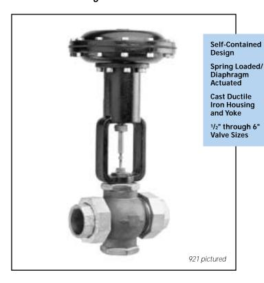
The Trerice Series 921 Pressure Regulator is fully self-contained and requires no external power source. This regulator requires that a user-supplied pressure sensing line be connected from the controlled point to the diaphragm actuator. Pressure in this line acts upon the diaphragm to develop the necessary thrust to stroke the valve, thereby maintaining the system at the desired condition.
