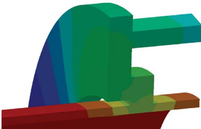
Temperature distribution on a floating ring assembly
