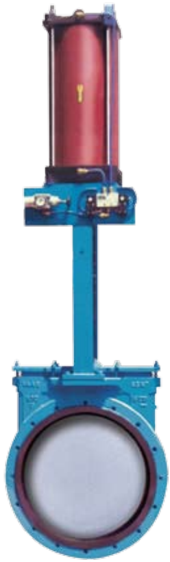
FIG 970 Coal mill isolation Knife Gate Valve complying to NFPA-85 (2001) design requirements featuring full flow bore and various hardfacing options for erosive boiler coal firing applications
