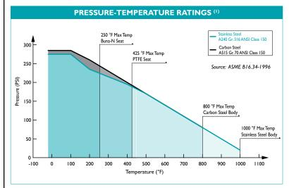
1. This chart displays the pressure-temperature ratings for the valve's body. Max temperature limits have been added for seat, body seal, and spring materials.
